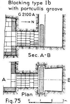
The portcullis slab stood upright against the masonry blocking and covered the rock-surface beside and above it. A number were pierced through the upper part with two or three holes obviously for the attachment of the ropes used in lowering the slabs. In five tombs in Cem. G 2100 the shaft had a rectangular groove at the southern end of the eastern and western sides down which the portcullis slab was lowered. The list of tombs with portcullis grooves is as follows:
