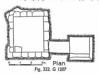
Passage: in rock, 1.7 × 1.25 m. and 1.45 m. high; length through lining, 2.1 m.; step down from floor of passage to paved floor of chamber, 0.45 m., and to rock, 0.7 m.
