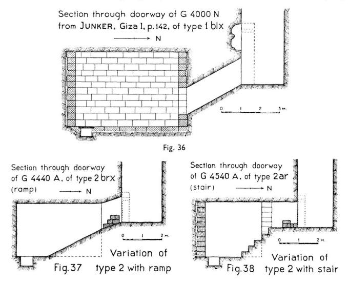
downwards. The floor of the doorway on the shaft side may be at the level of the bottom of the shaft or above it. When the passage is horizontal the type is designated as 1 ar, 1 am, &c. When the passage slopes down to the opening in the chamber, an 'x' is added to the type designation (type 1 arx, &c.). The designation 'x' combined with any type marks the connecting passage as sloping in some degree (Fig. 36).
