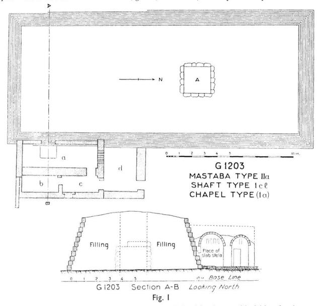
I b: A similar mastaba, filled solid (or more or less solid) with c.b., roughly laid as headers; private mastabas from the beginning of Dyn. III: both these types were plastered outside with mud which in turn was coated with white plaster.
