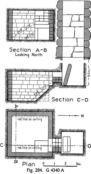
Shaft G 4340 A: 1.98 × 1.98 m.; -9.2 m. in rock; lined above with massive masonry, 5.0 m.; 6 courses.
