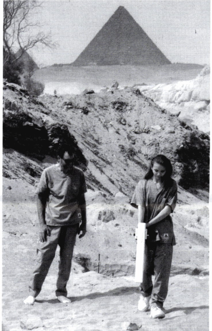
Gradiometer survey in progress. Becky Dash operates the FM 36 gradiometer while Glen Dash watches. Both wear surgical scrub suits because these clothes have no metal that could interfere with the survey equipment. Menkaure's pyramid rises in the background and at the right, the west end of the Wall of the Crow disappears under the sand.
