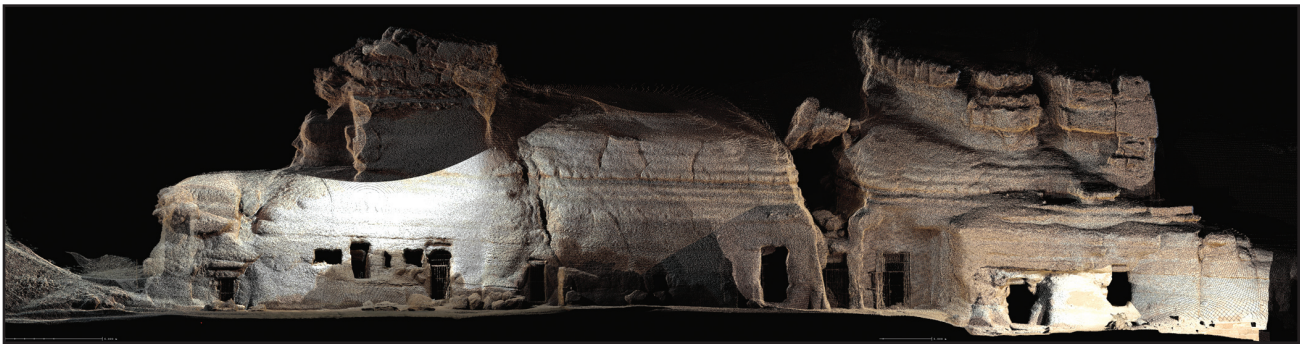
Plate 47.2. An orthophotographic point cloud image of the southern edge of the Moqattam Formation, which is north of the monument and adjacent to it, produced by the Riegl LMS-Z420i.
