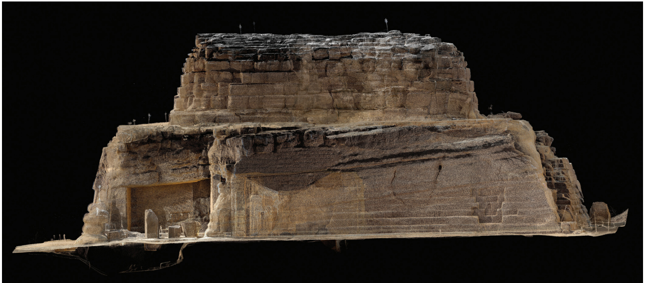
Plate 47.1. An orthophotographic point cloud image of the eastern face of the tomb produced by the Riegl LMS-Z420i.
