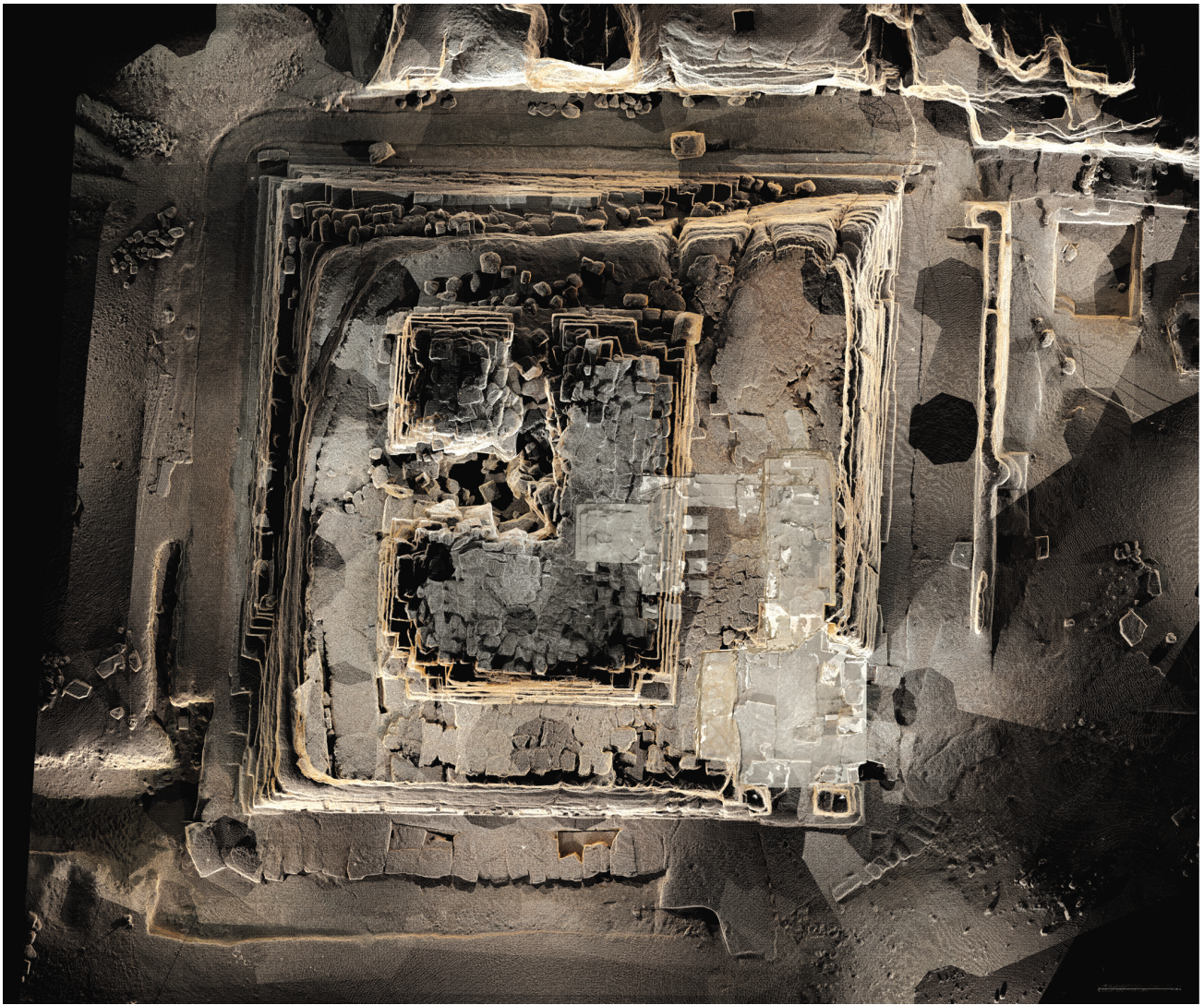
Plate 46.1. A plan of orthophotographic point cloud image of the tomb produced by the Riegl LMS-Z420i.
